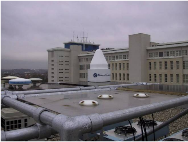
Figure 2. Space Engineering antenna mounted on the rooftop of the Septentrio office (Leuven-1). The site of Leuven-2 was chosen between the ventilation ducts similar to shown in the bottom right corner of this photo in order to get more short-range multipath.
