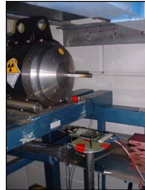
Figure 9: The PolARx2 below the Gammamat TK1000 at the test facility of FhG/INT, Euskirchen
