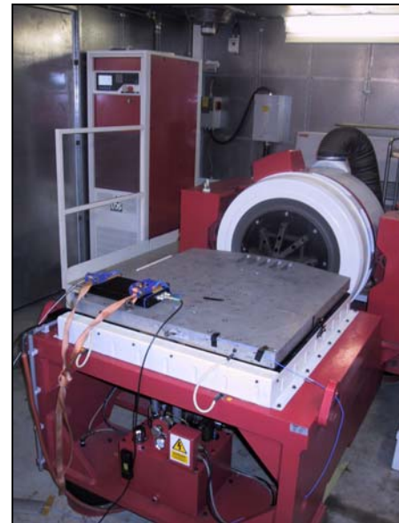
Figure 16: The PolaRx2 in the default housing on the electromechanical shaker
